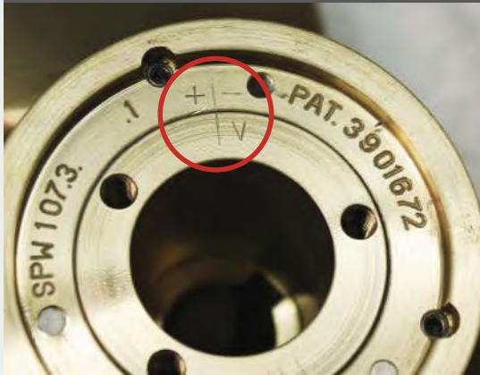
original factory pitch setting : markings line up
