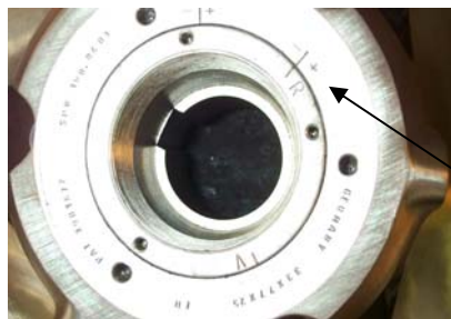
original factory pitch setting astern
