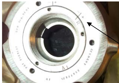
original factory pitch setting astern
