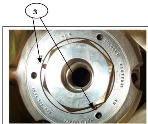
Carefully align the lock-pins (3) straight. They must go in easily. If not, try first to tighten the propnut a little further until they do. If impossible, back off the nut a little. The lock-pins should be hand tightened only. If overtightened they may strip.
