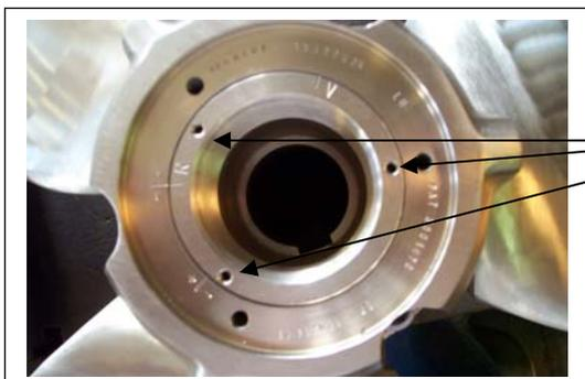
**Only two** of the three lock-pin holes can be used, depending on the final position of the shaft-nut flange ( 3 ).
