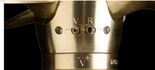
Marked lettering of a LH Propeller
