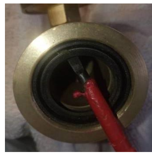
Remove the circlip with a slotted screwdriver
