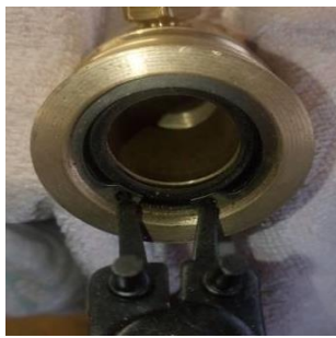
Remove the circlip with a circlip pliers
