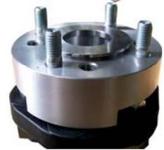
If required use a hammer and the beating wood to place the center ring correctly. But consider that you only little effort to press the center ring if it has been placed correctly before!
