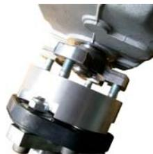
Now place the clamping flange on the shaft and make sure that it fits completely. Mark the position with a felt pen to make sure for the later assembly that the shaft is placed sufficing deep in the clamping flange. Make another mark 15mm to aft to control while assembling that the shaft has not been pushed too far through the clamping flange.
