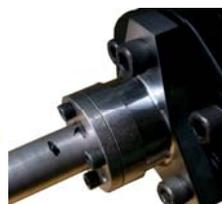
Now screw the screw nuts crosswise at the gearbox side with:
