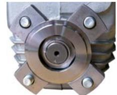
Place the center ring on the mounting surface of the coupling and press it into the coupling element.
