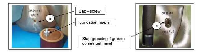
Factory supplied special grease EP/SAL is recommended and available from your VARIPROP distributor. Avoid regular white grease (sterntube-grease)!
