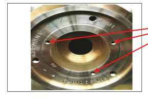
**Only two** of the three lock-pin holes can be used, depending on the <u>final position</u> of the shaft-nut flange ( **3** ).
